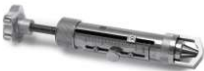
Gambar 11.2. Hardness tester (Sumber : (Murtini & Elisa, 2018))
