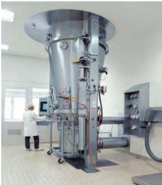
Gambar 6.6. Fluidized bed granulator (Sumber: Allen, 2014)
