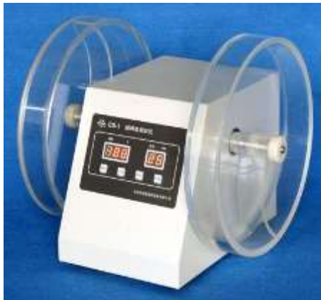
Gambar 11.3. Friability tester (Sumber : (Murtini & Elisa, 2018))
