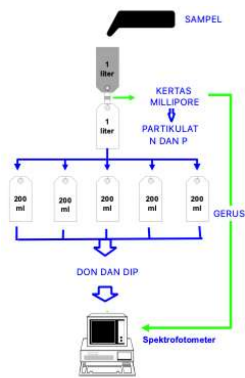
Gambar 5.2. Prosedur pengukuran sampel sampel limbah cair.
